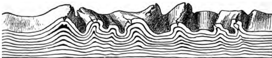
Fig. 54.—Showing the artificial folds produced in a series of layers of clay, on indiarubber, according to an experiment by Prof. A. Favre.
